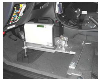
Force and way measurement of the brake pedal
